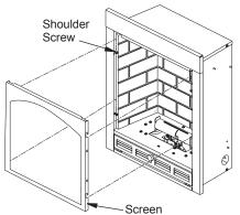
Figure 2 - Removing and Replacing Screen
